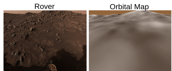
Fig. 2: High-level overview of the global localization framework. A) Transforming the rover images to match the orbital map: a 360 rover panorama of stereo images are radiometrically corrected, stereo matched, and orthographically projected into a 2D grid. B) Matching the rover images to the orbital map: the orbital map is cropped based on rover odometry’s position uncertainty, the orthomosaics are template matched to the orbital map based on the census and SSD similarity measures, and the best score is extracted and converted into a delta position update.
