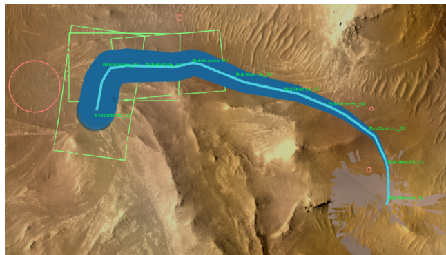
Figure 2. Demonstration of the onboard position uncertainty growth that occurs on long drives. A single set of drive instructions was sent to Perseverance on Mars to drive over multiple Martian days, sols 717-719. It drove 655.8 meters on Mars over that period, shown by the light blue line from the bottom right corner to the top left. The uncertainty, shown in dark blue, grew monotonically from 0 meters at the start of the drive to 32.92 meters at the end of the drive, because no global localization was performed during the three driving sols.
