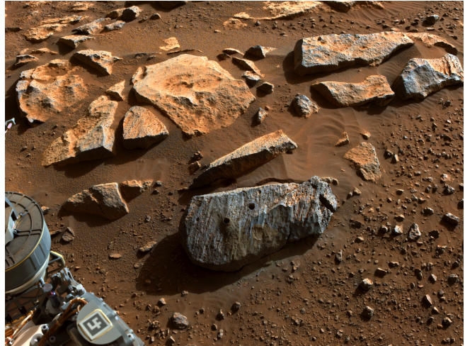
Figure 3. This Navcam image taken by NASA’s Perseverance rover on Sept. 7, 2021, PDT (Sept. 8, EDT), shows two holes where the rover’s drill obtained a pair of chalk-size core samples at the feature named Rochette.
