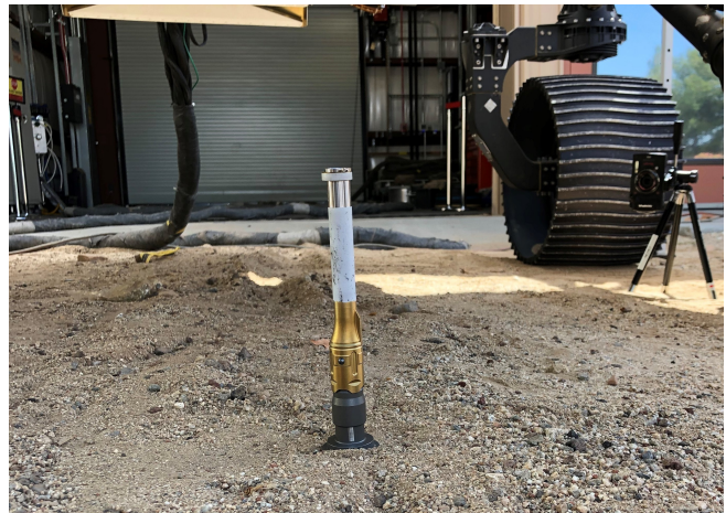
Figure 5. RGA resting vertically following drop to terrain in test.
