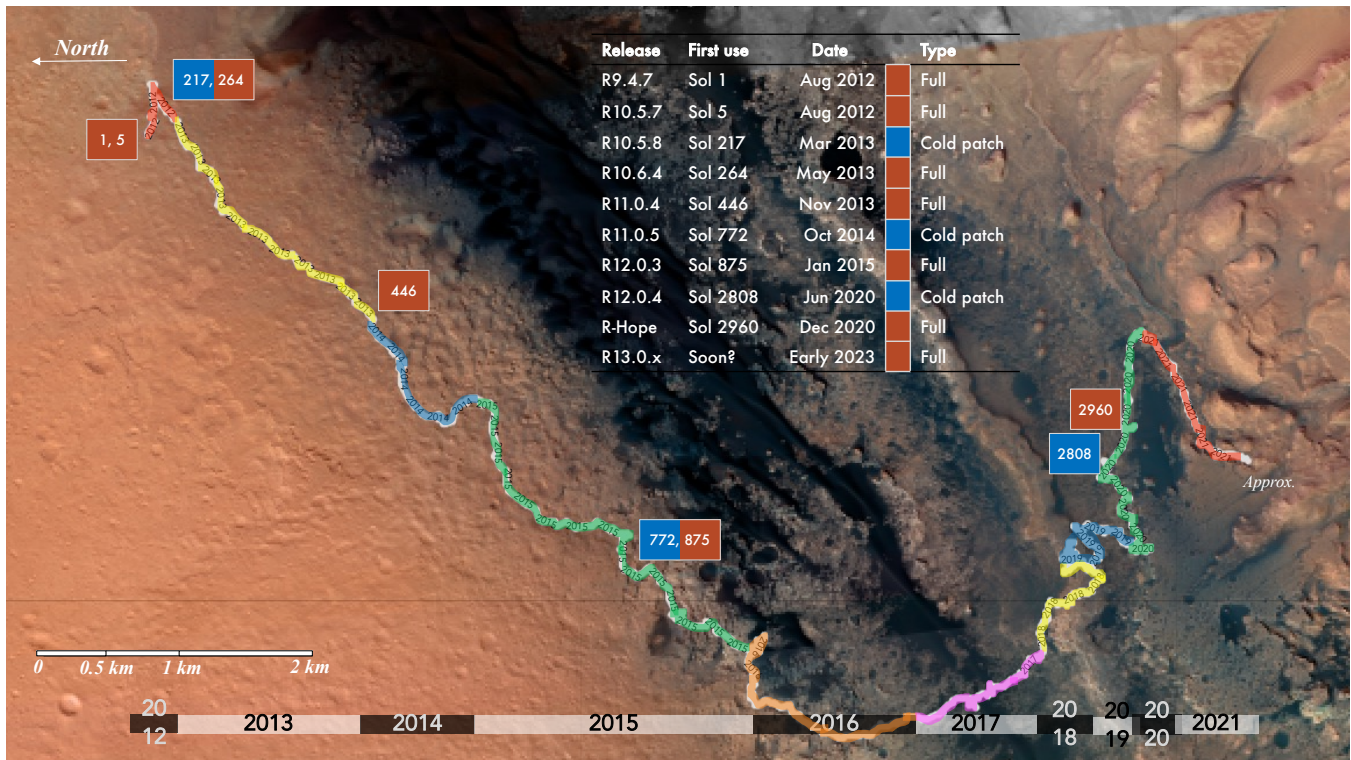
Figure 1. Flight software releases during the rover’s traverse, 2012 to 2021. More than six years have elapsed between R12, the last full flight software release for both prime and backup computers on sol 875, and the expected R13 release date. Full releases (orange); cold patches (blue); hot patches not shown. The colors on the dots indicating rover location are not meaningful, they just serve to indicate distinct Earth calendar years, which are labeled in the legend at the bottom of the figure.
