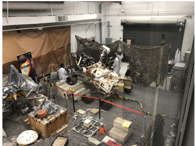
Figure 5. The Vehicle Systems Testbed performing testing at sloped attitudes inside the constraints of the In-Situ Instruments Laboratory at JPL
