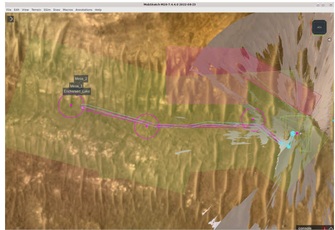
Figure 32. SSIm simulation results displayed in MobSketch (in blue). This is a screen capture, so the font size of target names appears relatively small here.
