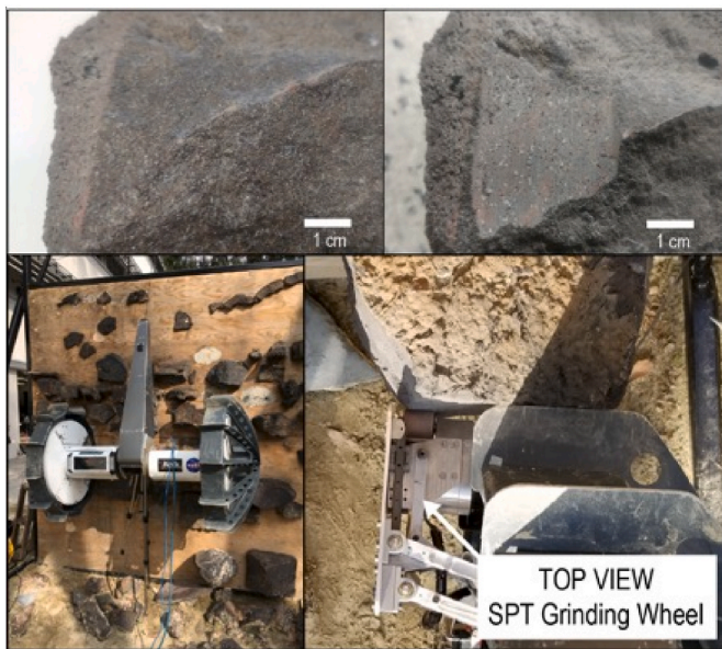
Fig. 18. Prototype of the SPT grinding a basaltic rock on a vertical wall using the Axel rover. ( top left ): basaltic rock with laser-rastered patina; ( top right ) fresh and flat after 15 min of SPT operation at 12 W and 5-N preload; ( bottom ) SPT's performance verified in a worst-case geometric configuration: only one wheel grouser in contact on a vertical wall.
