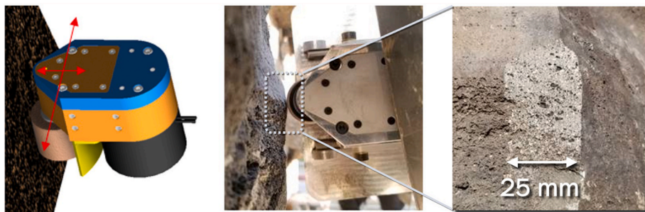
Fig. 7. Surface preparation tool design (left), prototype (middle), and result from grinding a basaltic rock on a vertical wall (right).
