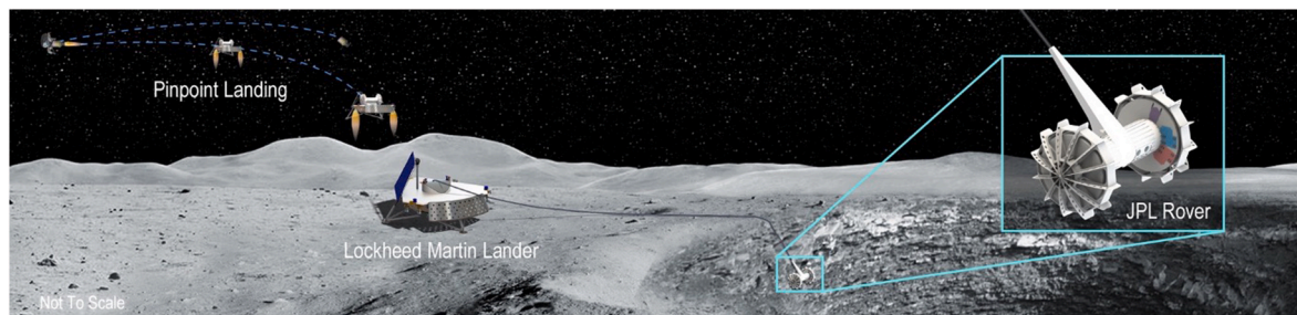
Fig. 1. The Moon Diver mission concept delivers a lander in the vicinity of the Mare Tranquillitatis pit and deploys a tethered rappelling rover with its instrument suite across the pit funnel and wall to acquire science measurements.
