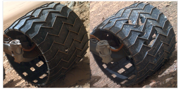
Figure 2: Rover wheel wear: Martian wheel photos on sol 490 (left) and sol 2030 (right), with significantly more damage visible in the later photo
