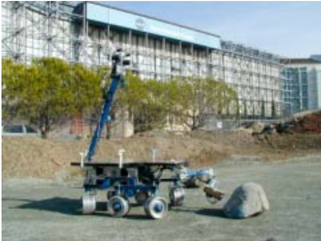
Figure 3 – The K9 rover places an instrument against a rock in the NASA Ames Marscape.
