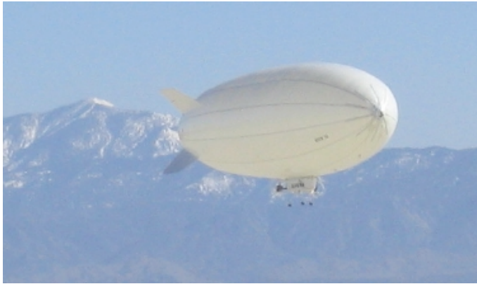
Fig. 7: Autonomous flight of the JPL aerobot, conducted at the El Mirage dry lake in the Mojave desert. The JPL aerobot testbed has a length of 11 m, a diameter of 2.5 m, and a static lift payload of approximately 12 kg.
