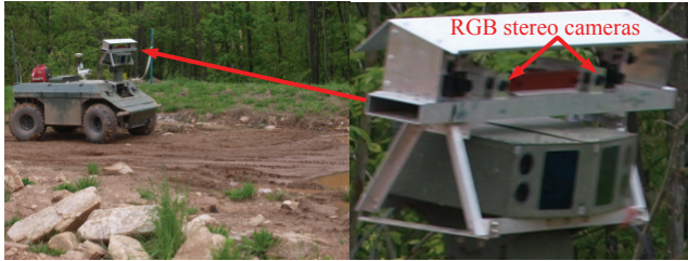
Fig. 1. JPL water detection software has been integrated onboard XUVs and evaluated at Ft. Indiantown Gap, PA. A forward-looking stereo pair of color cameras provides water cues from color, texture, and object reflections.
