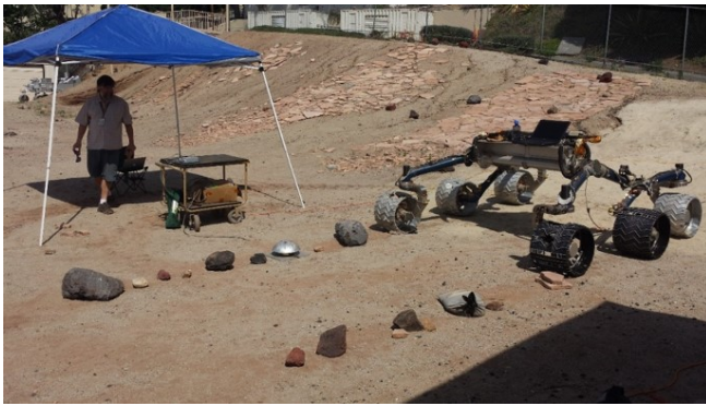
Figure 12. Complex terrain tracks used in Scarecrow development testing. The aluminum dome, which was mounted to the top of a load cell, is one of the objects driven over by the right wheels.
