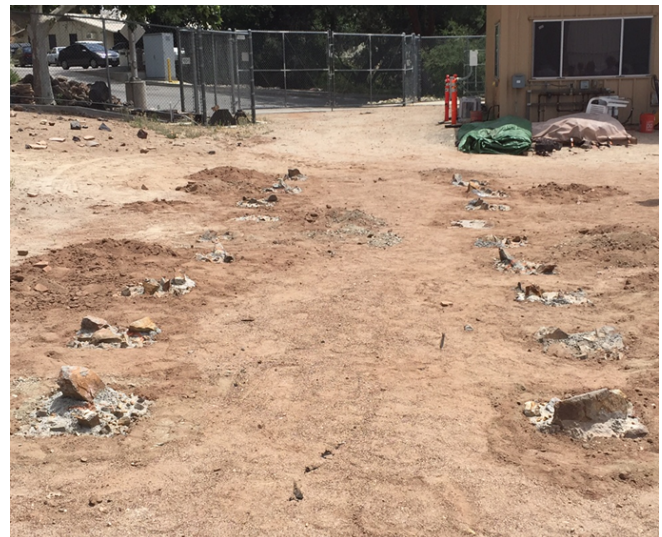
Figure 14. Complex terrain course constructed with high-friction, embedded rock tiles.
