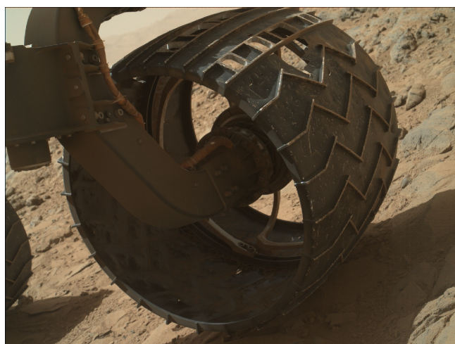
Figure 1. This MAHLI image, taken on Sol 490, depicts puncture damage on the left front wheel.
