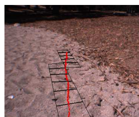
Fig. 1. Learning to correlate how things look to how they feel: the rover collects visual information about the forthcoming terrain from a sequence of stereo pair images, which is later correlated to the experienced slip at the locations traversed by the rover. An image from the left stereo camera displaying the rover’s future steps and the corresponding map cells (left), and the measured slip on the future path of the rover (right). Slip is measured as the difference between the commanded position per step (estimated by the vehicle’s kinematic model) and the actual position (ground truth), normalized by the commanded position.
