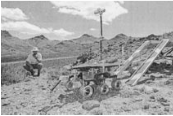
Fig. 2. FIDO rovers with the mast and instrument arm deployed at Black Rock Summit.
