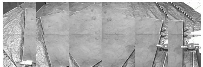
Figure 14 - Twelve left MCI images acquired by the workspace panorama command sequence. Two tiers of 6 images are acquired.
