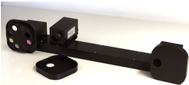
Figure 3 - The MCI testbed camera bar, with the right filter wheel cover removed. (DLR materials courtesy of: Ralf Jaumann, Nicole Schmitz, Frank Trauthan, DLR, Berlin)
