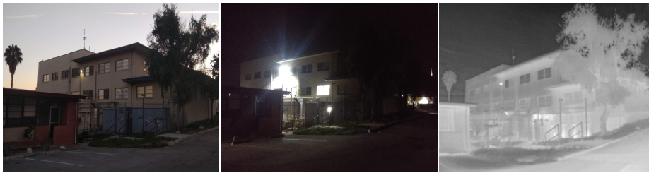
Fig. 1. An instance of a scene captured with visible-spectrum camera during the day (left), at night (right) and with a TIR camera at night (right). It can be seen that the nature of TIR modality enables the MAV to have more robust night vision.
