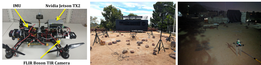
Fig. 3. (a) Quadrotor platform, (b) Test setup during the day, and (c) at night.
