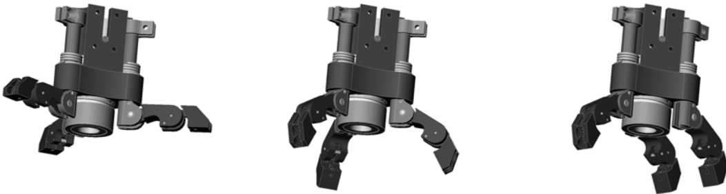
Figure 4. Gripper foot open, in the ball grasp configuration, and in cylinder grasp configuration
