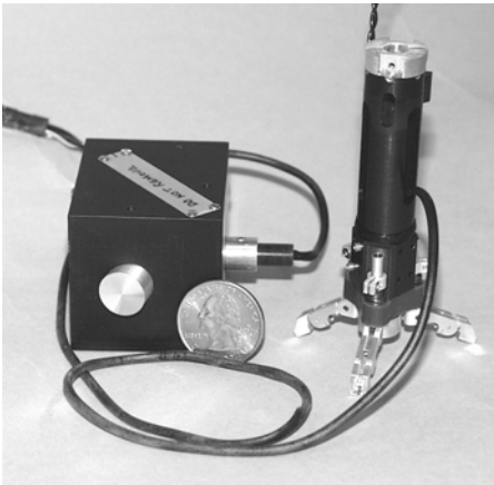
Figure 6. Full camera system with fore-optics incorporated into gripper tool
