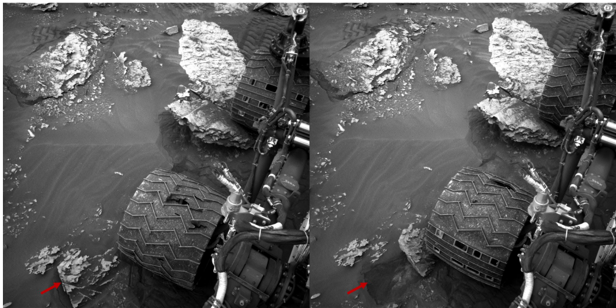
Figure 31: NavCam images of the RM and RR wheels on sols 2086 (left) and 2087 (right). The sol 2087 forward drive faulted when 98.7% wheel slip occurred, exceeding the 90% limit set for this drive. No forward progress was made. Note that a rock was dragged backward by the RM wheel.
