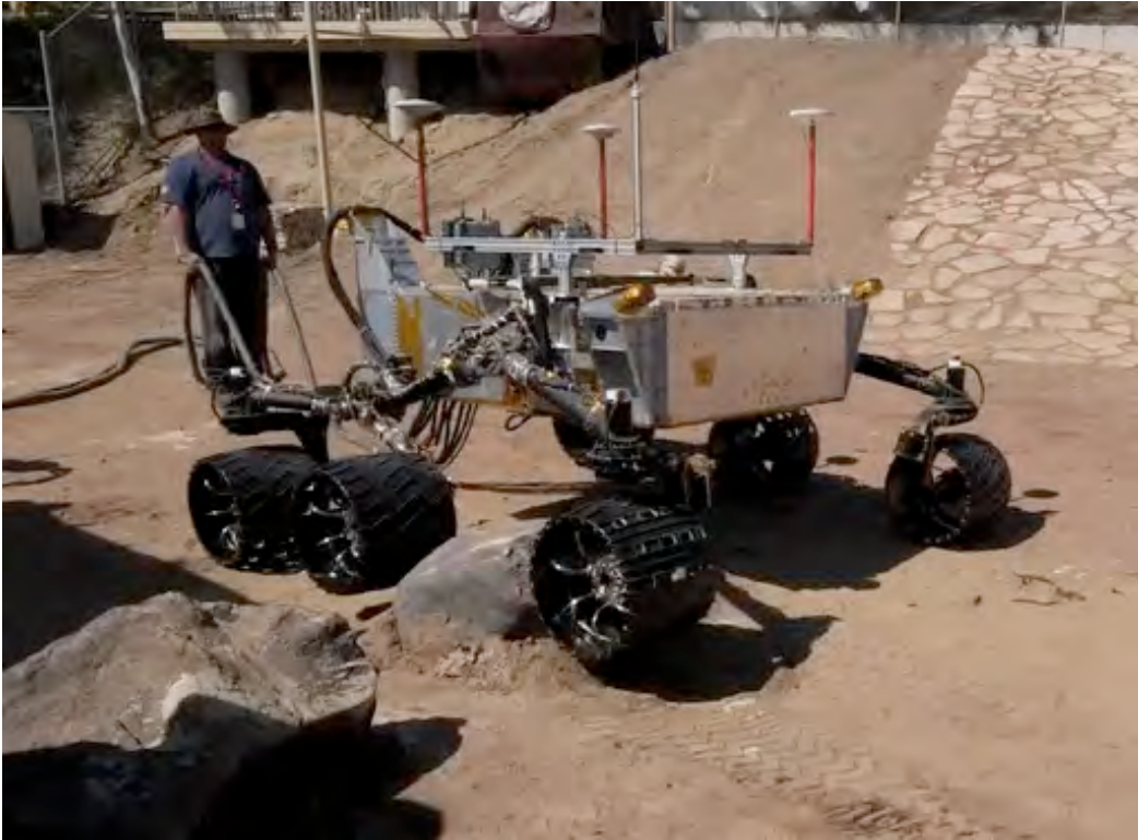
Figure 54: A 50 cm tall rock with a length of approximately 0.68 meters became wedged between the RF and RM wheels of the MSL Dynamic Test Model rover while driving backward over the rock.
