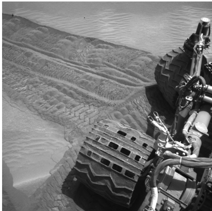
Figure 43: Sol 711 NavCam image of the RM and RR wheel after a turn-in-place command timed out. According to IMU data, the turn slip was 40.4%.
