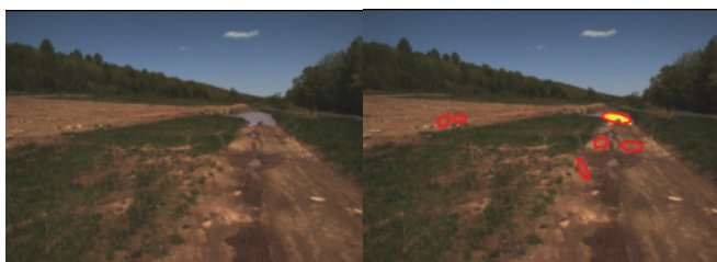
Fig. 10. A variety of characteristics are thresholded to detect water bodies based on color variation. Here, each red ellipse contains a single candidate water body. Only the one labeled yellow is ultimately detected as water.
