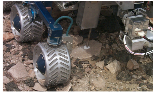
Figure 14. The miniature core drill acquiring a core sample from a carbonate rock at Silver Lake
