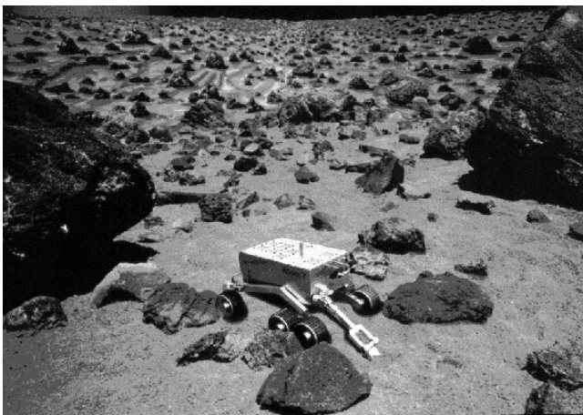
Figure 1. Rocky 7 Rover without solar panel in JPL Mars Yard
