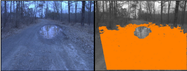
Figure 3. Ground detection around the boundary of a water body is used to estimate the elevation of the water body.
