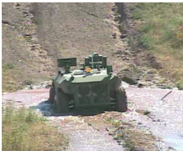
Figure 1. An experimental unmanned vehicle (XUV) navigating on a flooded portion of a road on a test range at Ft. Indiantown Gap, PA.
