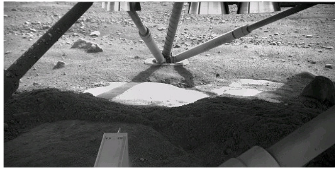
Figure 17 — The RA positioned the RAC to take this image of the back footpad by looking underneath the Lander to support assessment of Lander stability
