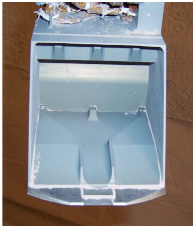
Figure 4 – Scoop interior showing the channel used to guide the material sample when delivering to the TEGA and the MECA
