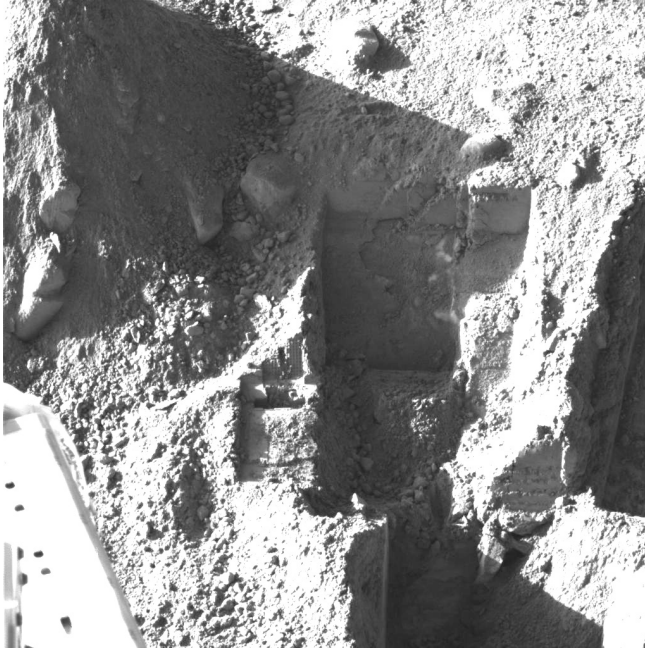
Figure 16 — The SSI captured the state of the Dodo-Goldilocks trench before and after the cave in experiment on sol 116 clearly showing the impression made by the scoop and material in the trench
