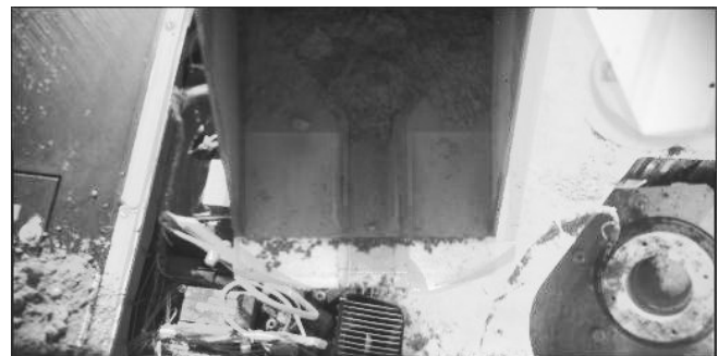
Figure 12 – This image consists of two overlaid RAC images of the scoop posed over MECA WCL 0 ready for delivery on sol 29 - one from Mars and the other from the PIT
