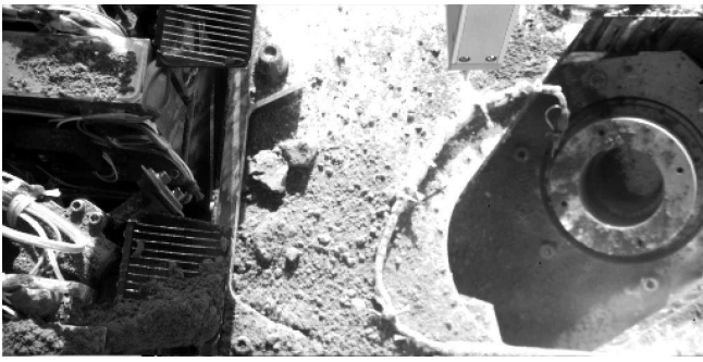
Figure 13 — The RAC took this image shortly after the RA delivered a sample from Rosy Red to MECA WCL 0 (lower left cell) on sol 66 verifying successful delivery
