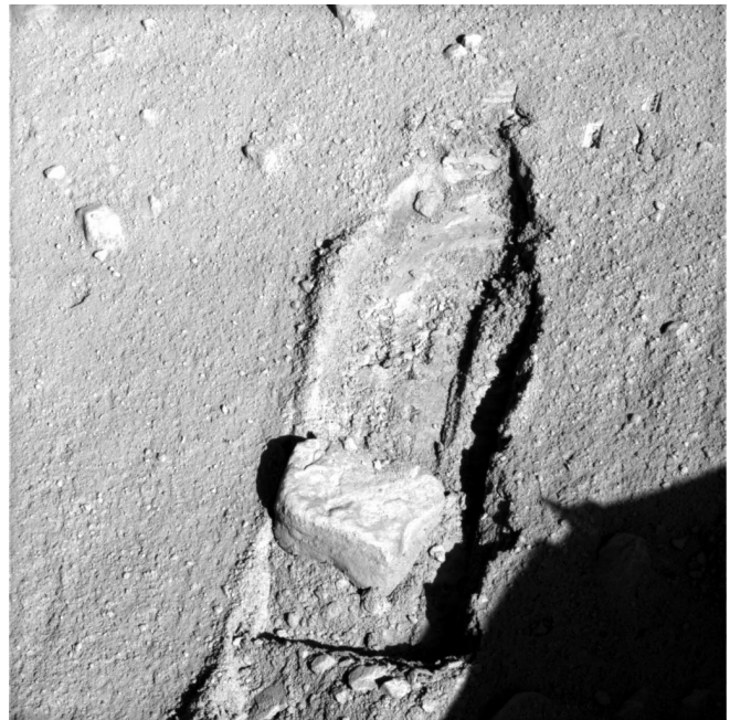
Figure 15 — On sol 117 the RA pushed a rock 0.5 m into a trench excavated below it using the scoop to reveal the surface underneath
