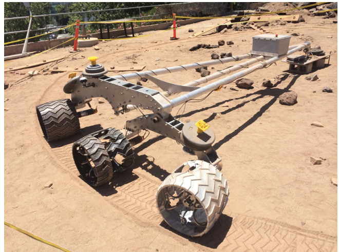
Figure 28. Wheel life testing was performed in the JPL Mars Yard using a three-wheel test rig with rocker and bogie suspension arms and a front, middle, and rear wheel. Image Credit: NASA/JPL-Caltech
