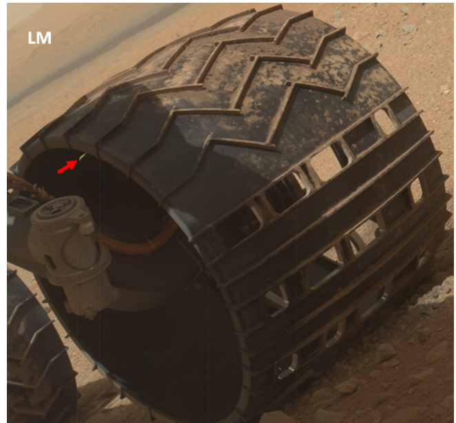
Figure 6. Cropped sol 34 MAHLI image of the LM wheel showing the first observed damage to Curiosity wheels. Image Credit: NASA/JPL-Caltech
