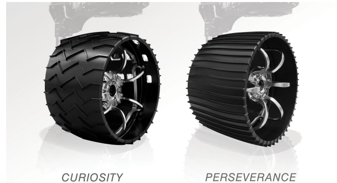
Figure 30. Side-by-side view of a Curiosity and Perseverance wheel. Image Credit: NASA/JPL-Caltech.
