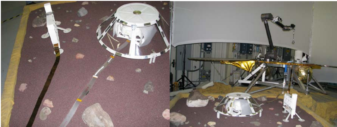
Figure 17 Manually selected SEIS/WTS and HP3 placement during the site visit.
