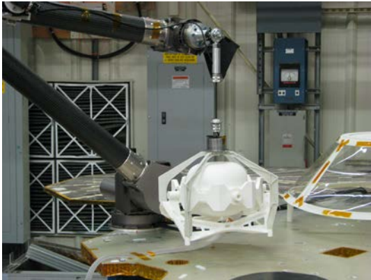
Figure 6 - COTS prototype magnetic grapple on a 20 cm umbilical lifting a mass and volume mockup model of SEIS off the Phoenix flight systems testbed Lander.
