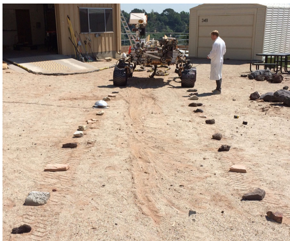
FIGURE 8 TRCTL testing in the JPL Mars Yard on the VSTB testbed. One of the objects driven over on the left side is a ground anchored FTS with an aluminum hemisphere dome mounted on top of it. FTS, force-torque sensor; JPL, Jet Propulsion Laboratory; TRCTL, our algorithm inspired by traction control; VSTB, Vehicle System Testbed [Color figure can be viewed at wileyonlinelibrary.com ]
