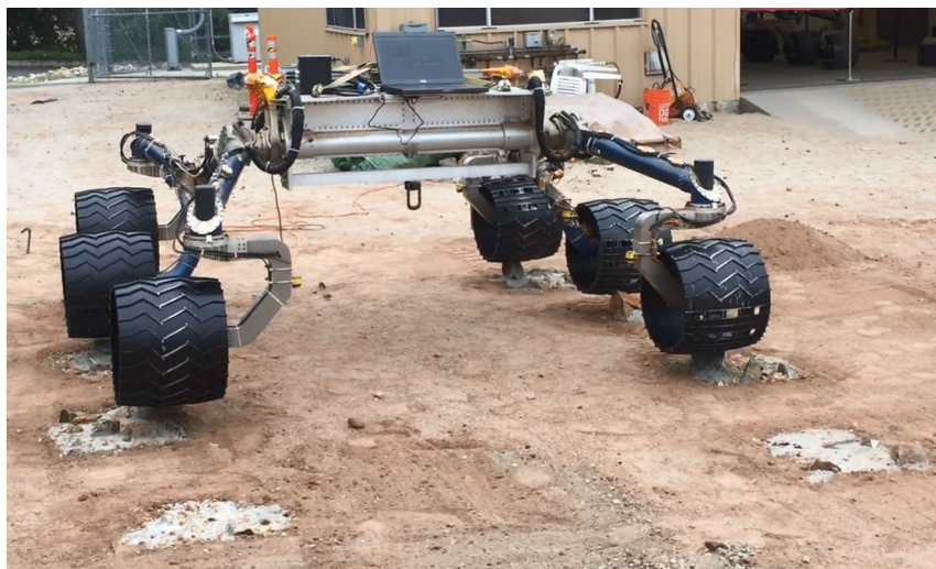
FIGURE 9 The Scarecrow testbed rover on a complex-terrain test course in the JPL Mars Yard. Eighteen cement tiles containing embedded rocks were installed at 1 m intervals along the paths of the wheels. The tile spacing on the left and right sides was the same to prevent wheels from missing some tiles due to yawing off course. JPL, Jet Propulsion Laboratory [Color figure can be viewed at wileyonlinelibrary.com ]
