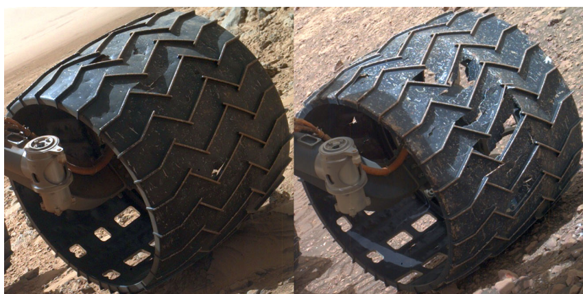
FIGURE 1 MAHLI image of the Left Middle (LM) wheel on Sol 490 (left) and Sol 2030 (right). In the Sol 2030 image, one of the two LM grouser breaks is visible. MAHLI, Mars Hand Lens Imager [Color figure can be viewed at wileyonlinelibrary.com ]
