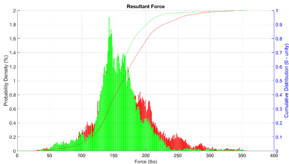
FIGURE 10 Cumulative frequency distribution of resultant loads on Scarecrow RR wheel during traverse of high friction, embedded rock tiles. Green and red correspond to TRCTL enabled and disabled, respectively. TRCTL, our algorithm inspired by traction control [Color figure can be viewed at wileyonlinelibrary.com ]
