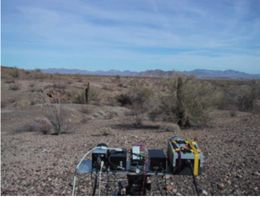
(a) Color image of scene and sensor setup. Two NC256 MWIR and one LWIR cameras were used.
