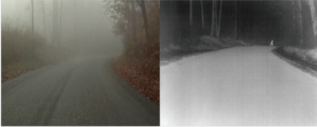
Fig. 37. Color and Photon LWIR image of a scene containing fog. A pedestrian is obscured by the fog in the color imagery but is evident in the LWIR image.
