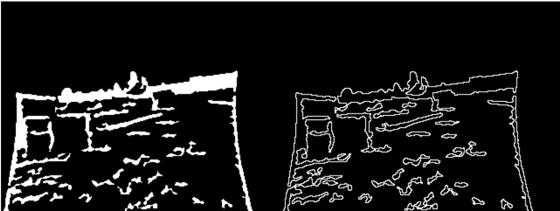
Fig. 5. The left image contains potential negative obstacle regions following the filtering in Figure 4 and removal of all regions smaller than 50 pixels. The right image is a closed contour image of the candidate negative obstacle regions.
