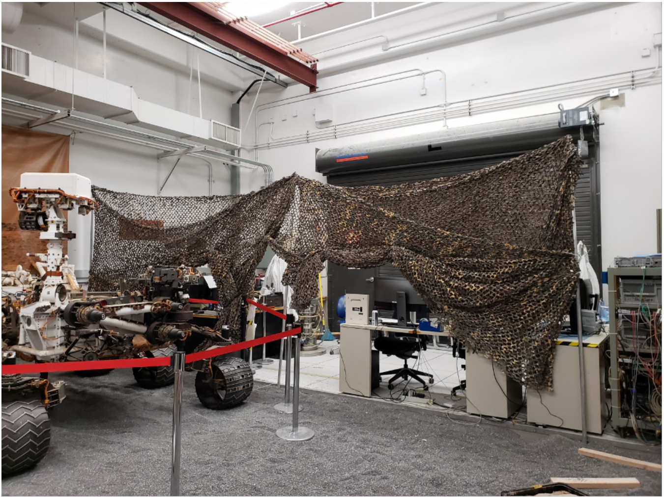
Figure 10. VSTB in ISIL with camouflage tarp to ensure VO convergence
