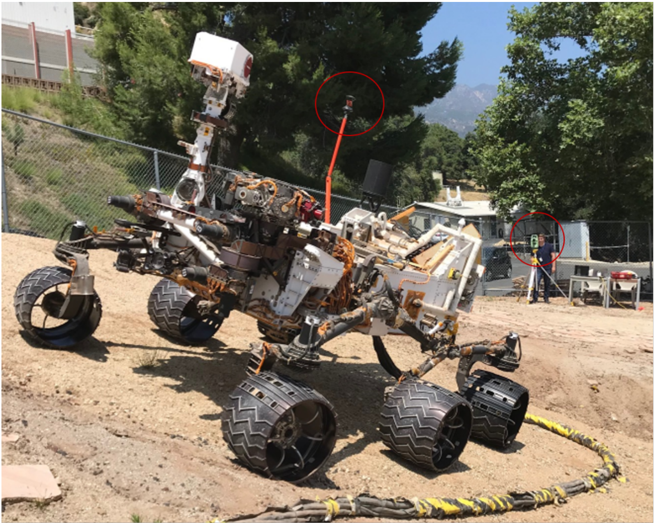
Figure 7. VSTB in the Mars Yard with Total Station Tracking System
