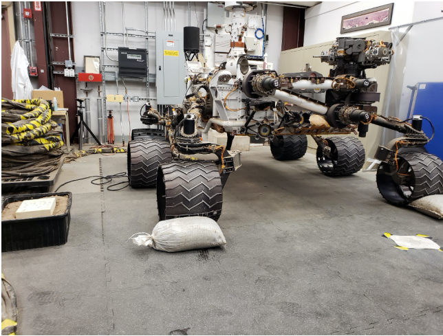
Figure 8. A sandbag is placed in front of each front wheel prior to a forward drive to induce a suspension fault response.
